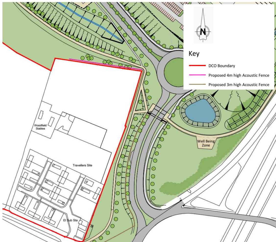
Figure 1.1: A47 Link Road and Acoustic Barrier Locations
